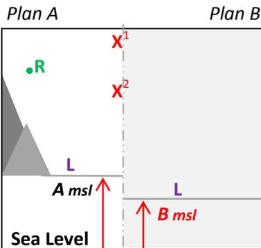
As shown in side view at left, Plan A assumes a closed course using a Start/Finish Point at the home airport; in contingency Plan B, the glider lands out after achieving the Start and one or more Turn Points in the shaded area. In this case...
