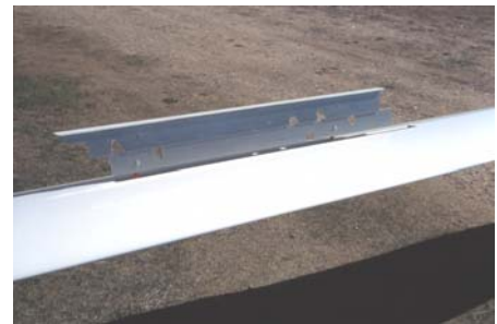
Spoilers come out of the wing and create drag for landing. Image by Bill Hoadley
