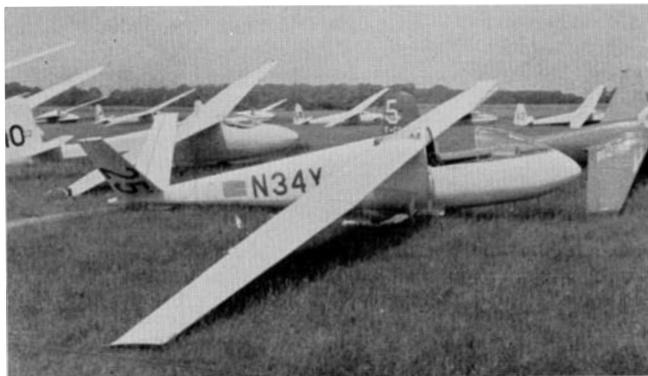
The two Polish Zefir 2's entered in the open class. Wing tip booms on #14 supposedly carried thermal sensing devices. Retractable wheel, no skid.
